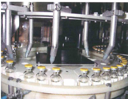
fig. 3: Removal of residual water by pressurized air.
