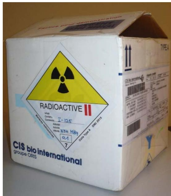
Figure 13.7 Exemple de colis Type A
